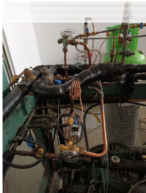
Figure 5. Compensator bridge for R404A and R22 TXV (right) and TXV
